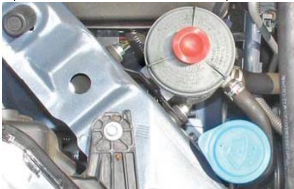
This is the original design on the reservoir. Note the location of the ribs to determine if this is the older or newer style.
